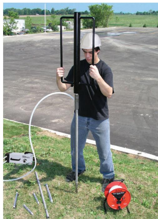
**Note:** for higher resolution profiling, Solinst offers the Model 660 Drive-Point Profiler, which can also be used with the Model 410 Peristaltic Pump. Samples are taken at multiple depths, as the Drive-Point Profiler is advanced deeper.
